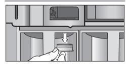
Pull the rubber connector down and out.
